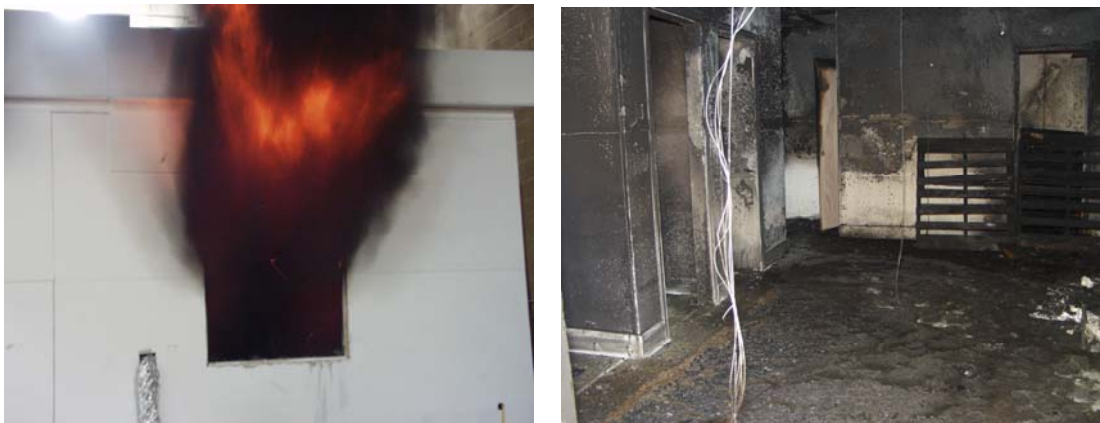
Figure 5. Test 2, exterior view of fire room during flashover and post test interior of fire room.
